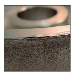
Worn-out, chipped off or scratched CBN coatings on the grinding surface or on the edges.
