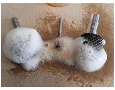
Spray the clogged areas with resin solvent (e.g. No. 705524 or 705599) and allow the agent to take effect (Fig. 2) - for several hours depending on the degree of clogging.
