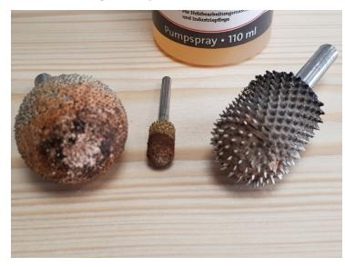
Depending on the nature of the wooden material (resin content, wood moisture, etc.) and your individual working methods, the spaces between the TC tips can become clogged with wood fibres or resin (Fig. 1).
