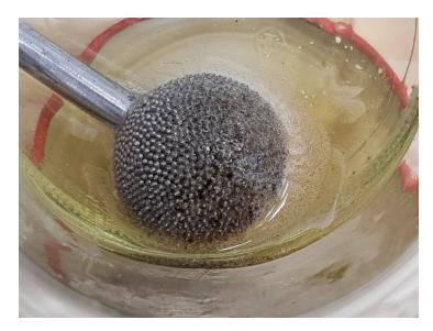
In the case of heavy clogging, repeat the procedure until the gaps are clear again. Alternatively, the burrs can be soaked in the resin remover for several hours (Fig. 3) to soften the dirt.
