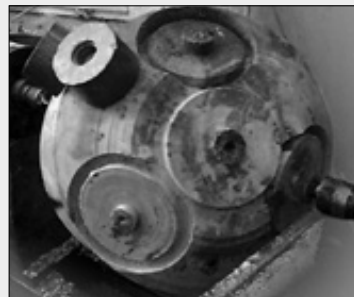
3 Three spigots with a diameter of 100 mm for the chuck are turned on the conical end of the blank.
