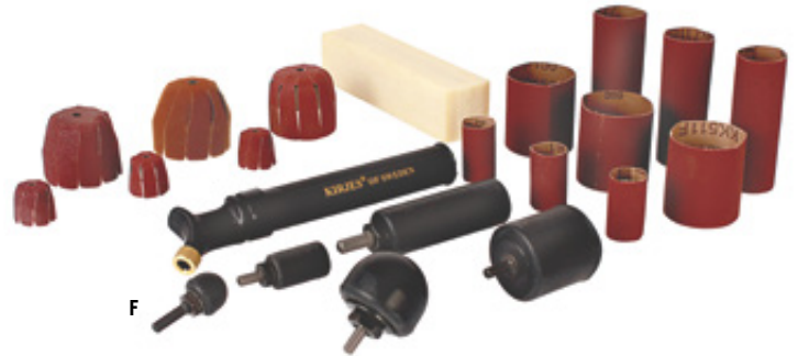
F DRUM SANDING KIT NO. 101 FOR KIRJES® SANDING SYSTEM Set includes: drum sander, Ø 20 x 32 mm (No. 120); drum sander, Ø 28 x 80 mm (No. 130); drum sander, Ø 42 x 44 mm (No. 140); dome sander, Ø 42 x 35 mm (No. 140R); dome sander, Ø 20 mm (No. 120R); one sanding sleeve (grit 80, 150 and 320) for each sander; hand pump; cleaning stick. No. 707435
