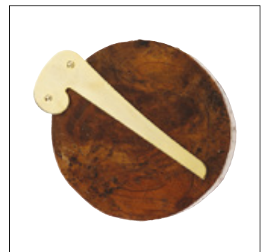
E CENTRE FINDER FOR ROUND STOCK Makes work fabulously easy: Simply place it on the end of a round piece of wood and mark two lines - the point of their intersection is the exact centre. Maximum Diameter of workpiece min. 20 mm / max. 220 mm. Length 130 mm No. 707262
