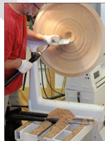
C LARGE OUTBOARD ATTACHMENT FOR ONEWAY 2436 LATHE Solid outboard attachment for a spindle height of centre over bed of 610 mm. Fits No. 705552 and No. 705549. No. 706538
