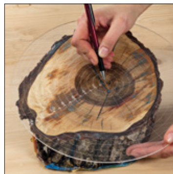
D CENTRE FINDER WITH CIRCLE Find the most beautiful centre of your turning blank.: Conventional centre markers find the geometric centre of a workpiece; the turned circumference is then aligned with this centre. However, especially with asymmetrical blanks (e.g. green wood blanks), a centre is sought that avoids defects and retains the visual highlights of the blank. Place the template and select the size and location of the surrounding area that will determine your centre point. An ingenious tool especially suitable for turning bowls with natural edges, burls, roots and eccentric workpieces. Diameter 300 mm Length 130 mm No. 702500
