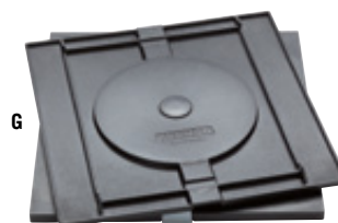
G TORMEK® ROTATING BASE Enables you to easily rotate the machine 180° and lock it with complete stability. It makes it easy to alternate between sharpening/honing or sharpening towards or away from the edge. Fits all models. No. 705221
