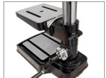
Height adjustment of the table by a trapezoidal threaded spindle integrated in the column, thus no toothed rack getting in the way.
