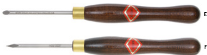
E HENRY TAYLOR® COVING TOOL For cutting coves in spindle and faceplate work to produce decorative patterns in combination with the texturing tool. Handle length 175 mm Blade width 6.5 mm Overall length 275 mm No. 702037
