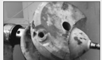
4 The three spigots having been finished, the blank is mounted on the chuck with one of these spigots. It now follows pre-drilling and blind-hollowing with a 13 mm spindle gouge. Afterwards, the outside of each part can be turned (not completely round) dividing the original bell form into three parts.
