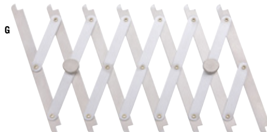
G M. POWER TOOLS POINT.2.POINT For laying out equal spacings, e.g. dovetails, dowels, etc. Extends to 600 mm and can be locked in any position to transfer up to seven position markings (six equal spacings) to the workpiece. Stainless steel, brass screws. Not suitable for high-precision applications. Max. length 600 mm No. 707267
