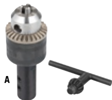
A SCROLL CHUCK 6.5 MM For mounting on the right-hand shaft. Comes with chuck key. For machine shafts with diameter 10 mm. Clamping range 1-6.5 mm. Bore 10 mm No. 728799
