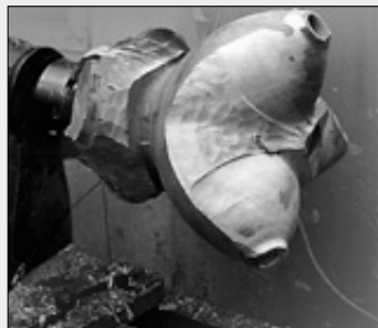
5 All three parts have been turned. The waste material is removed from the lower part of the blank with an Arbortech Industrial Pro blade mounted on an angle grinder. The spigots, however, remain.
