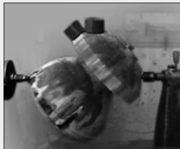
2 The blank is mounted between Centres again, this time, however, on diagonally lying points. On this and the following photos you can see, that heavy blocks of lead have been securely screwed onto the blank to bring it into balance.
