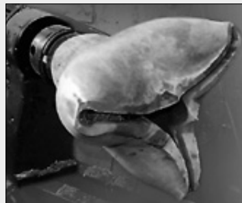
7 Now, the lower part of the object, on which it will later stand, is remounted and turned. The final star-shaped opening is cut with the Arbortech Industrial Pro blade. The roughly sanded vessel is then set aside to dry. Since the walls are approximately 5-6 mm thick, the danger that cracks will develop is relatively low.
