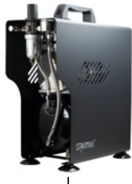
I SPARMAX® COMPRESSOR TC-610H PLUS Mid-range compressor for versatile airbrush applications: Small single piston compressor with 2.5 litre pressure tank and two hose couplings. Due to the air supply in the tank, it is also possible to work without a power supply for a short time (approx. 1 minute, depending on air consumption). The functional metal housing provides optimum protection for the pressure regulator, water separator and accessories, yet is lightweight for mobile use. Incl. water separator for clean and dehumidified air, removable pressure regulator with pressure gauge, automatic on/off function at 2.8 / 4.1 bar.
