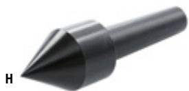
H LIVE CENTRE, #2 MT Revolving lathe tip with point angle 60°. Morse taper #2 MT Ø 30 mm Overall length 108 mm No. 714159
