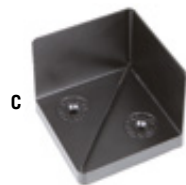
C VERITAS® CENTRE MARKER For easy finding and marking the centre of any round or square blank of up to 150 mm in diameter or across. You fix the marker to the wall, and tap the blank with a hammer. The result is two scoring lines that intersect at the exact centre. 80 x 80 x 70 mm. No. 707312
