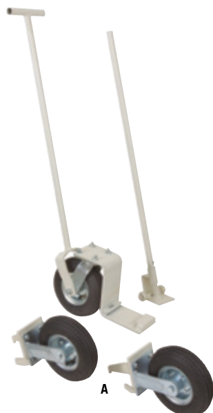
A WHEEL SET FOR ONEWAY 2436 LATHE, 3-PIECE SET Robust pneumatic wheels, comes with pry bar for lifting the lathe. The pneumatic wheels make it easy to move the heavy machine over ridges and uneven floors. Two fixed wheels and one for steering. The wheels are only intended for moving the lathe - they must be removed when turning. Fits No. 705552 and No. 705549. No. 706540
