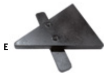
E SORBY™ PROEDGE GRINDING JIG, 45° FOR SKEW CHISELS This jig is placed onto the Sorby ProEdge support table. It allows you to grind a 45° angle without time-consuming angle setup and measurement. No. 720392
