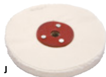
J SORBY™ PROEDGE POLISHING WHEEL Fits Sorby ProEdge. The cotton fabric, in combination with polishing paste No. 720397, creates a great polish for steel. Mount No. 720395 is required to use this product. Ø 100 mm Width 10 mm Centre hole Ø 10 mm No. 720396
