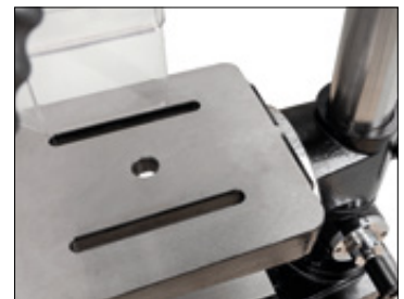
The machine table is tiltable by ± 45° and has two grooves for fixing the devices. It can be rotated 360° around the column.
