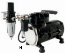
H SPARMAX® COMPRESSOR TC-501N Mini Compressor: Single piston mini compressor without pressure tank, also ideal for mobile applications. The integrated water separator cleans and dehumidifies the compressed air and ensures the finest spraying results. Oil- and maintenance-free air compressor incl. removable pressure regulator with pressure gauge, automatic on/off function at 2.8 / 4.1 bar.
