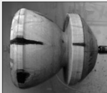
1 First of all, the woodturner develops a bell form eliminating a lot of weight. Then he turns a spigot with a diameter of 100 mm on the tailstock end, which is to be clamped in the solid chuck. Now the middle can be hollowed out.
