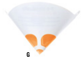
G DISPOSABLE FILTER, 25-PIECE SET Disposable paper filter with glued-in nylon filtering fabric. For filtering lacquers (Clourethan, Herdim dry spirit varnishes) and oil lacquers (Le Tonkinois). Top diameter 160 mm. Mesh opening 260 µm. No. 706149
