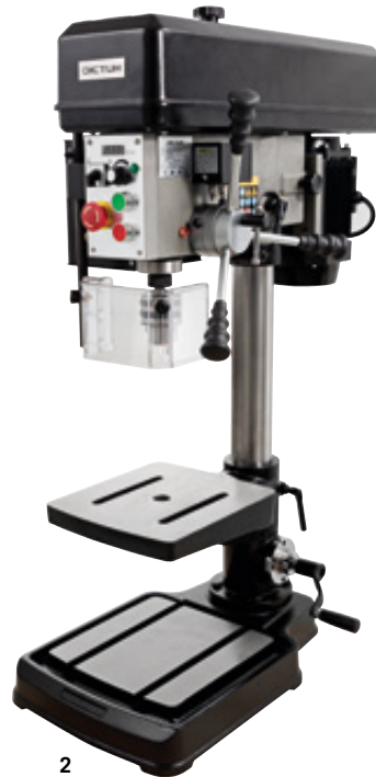
The machine table is tiltable by ± 45° and has two grooves for fixing the devices. It can be rotated 360° around the column.
