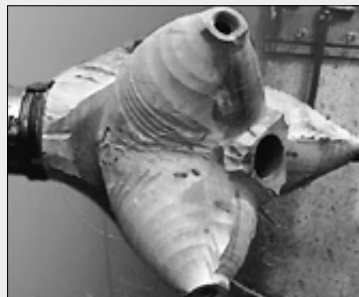
6 The photo of the completed object shows, that lips surround the star-shaped opening. Because of these lips the parts could not be turned round but have to be routed. The material which will form the lips must be left over.
