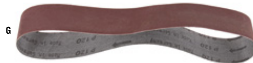
G SORBY™ PROEDGE ABRASIVE BELT, ALUMINIUM OXIDE This aluminium oxide abrasive belt is suitable for all HSS and carbon steels, such as chisels, plane blades, sculpting and turning tools. Dimensions 780 x 50 mm. Fits Sorby ProEdge No. 720384 and 720383. Grit 60 No. 701730 120 No. 720386 240 No. 720385
