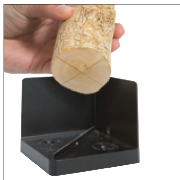
C VERITAS® CENTRE MARKER For easy finding and marking the centre of any round or square blank of up to 150 mm in diameter or across. You fix the marker to the wall, and tap the blank with a hammer. The result is two scoring lines that intersect at the exact centre. 80 x 80 x 70 mm. No. 707312
