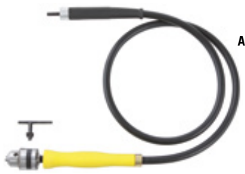
A FLEXIBLE SHAFT FOR KIRJES® SANDING SYSTEM Highly flexible, equipped with three capsuled ball-bearings and scroll chuck 0-10 mm. Intended for max. speed 10 000 rpm. Length 130 cm. No. 707433
