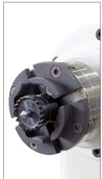
G SORBY™ STEB CHUCK DRIVER Saves time and effort: The Sorby Steb Chuck Driver can be easily placed and clamped on your current chuck. The need for time-consuming modifications is gone. Fits chucks Talon No. 702159/60 and Stronghold No. 702158, Super-NOVA2 No. 720670/71 and 720753. Overall length 50 mm Ø 13 mm No. 720377 22 mm No. 720378 32 mm No. 720376
