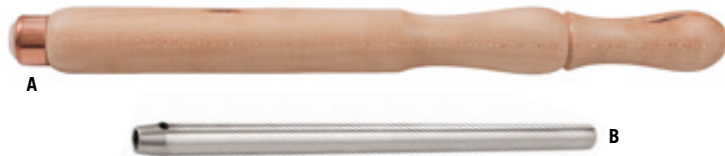
A MARTEL HARDWOOD HANDLE Oiled maple handle. Two handle surfaces for effortless and safe guidance of the tool. Fits No. 729641. Shaft 12.7 mm. Overall length 457 mm. No. 729644
