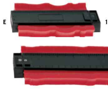
E PROFILE GAUGE WITH PLASTIC BLADES For measuring and transferring profiles. No offset necessary, as blades are flush with the frame. Blade thickness 1.3 mm.
