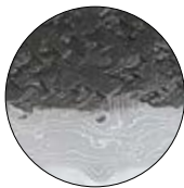
Lightly hammered surface with black forged skin
