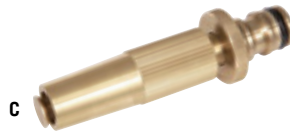
C GEKA® HOSE NOZZLE, BRASS, ½ INCH The water pressure of this brass nozzle can be continuously adjusted simply by turning the head. Suitable for ½-inch hose couplings, ideally with a water stop. Overall length 100 mm No. 746218
