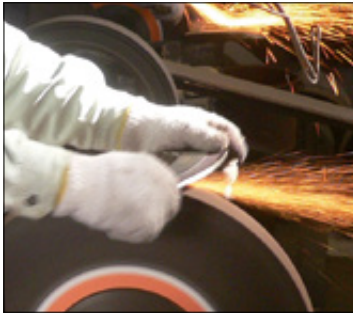
Form grinding of the forged blade
