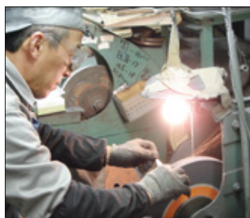
Coarse grinding of the flanks (bevel) on a grinder
