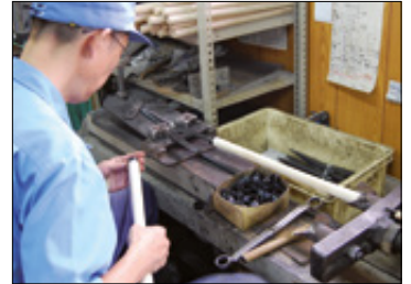
Assembly of the handles and bolting
