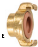
E GEKA® QUICK COUPLING FOR TAP, ¾ INCH, BRASS, DRINKING WATER The brass coupling for taps is suitable for drinking water and can be quickly connected to the quick couplings by means of a bayonet fitting. Suitable for taps with 26.5 mm DN 20 thread and all Geka quick couplings with 40 mm claw distance. No. 746220
