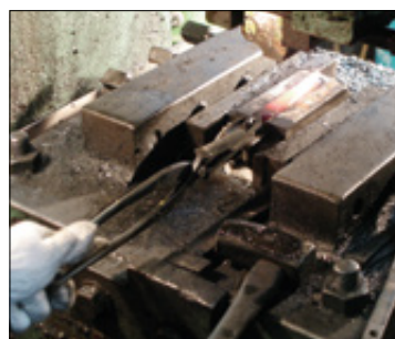
Forging of the shear blades
