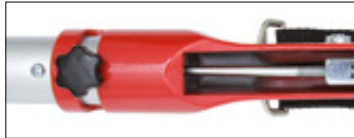
Ball valve of centre oiler
