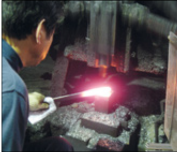
Forge-welding of the two steel layers
