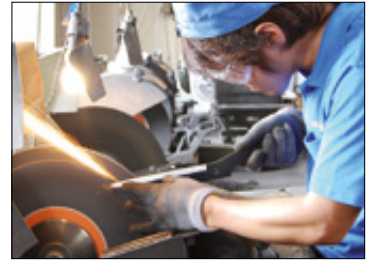
Pre-grinding of the shear blades after forging
