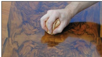
Polishing of shellac surface
