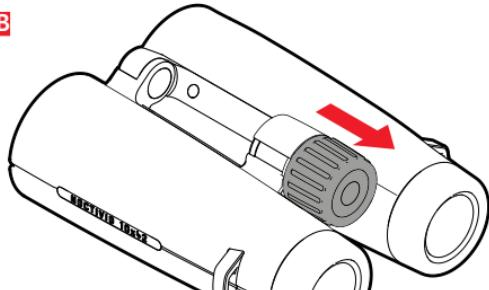
Next, pull the central focusing unit's wheel up slightly (Figure **B**).
