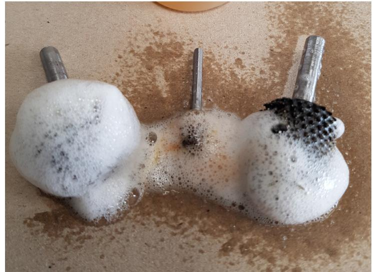
Spray the clogged areas with resin solvent (e.g. No. 705524 or 705599) and allow the agent to take effect (Fig. 2) - for several hours depending on the degree of clogging.
