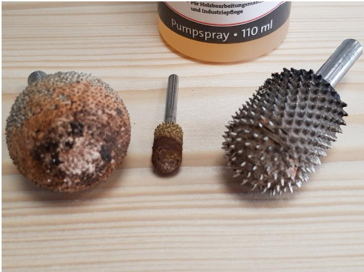
Depending on the nature of the wooden material (resin content, wood moisture, etc.) and your individual working methods, the spaces between the TC tips can become clogged with wood fibres or resin (Fig. 1).
