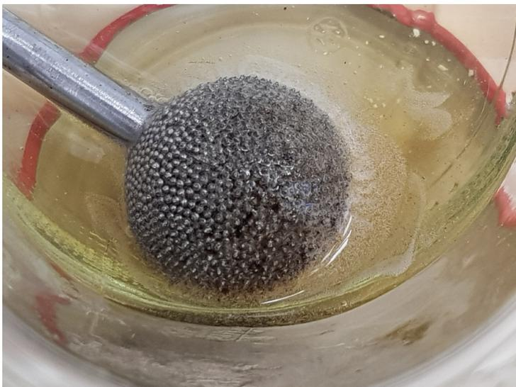
In the case of heavy clogging, repeat the procedure until the gaps are clear again. Alternatively, the burrs can be soaked in the resin remover for several hours (Fig. 3) to soften the dirt.
